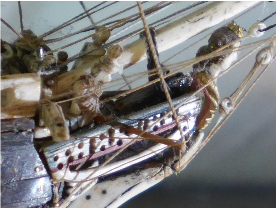
Pair of knightheads (left) and figurehead
