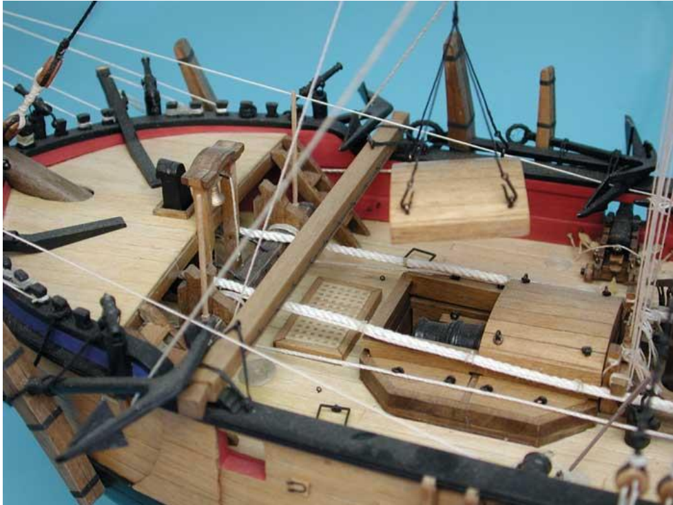
Wood model 5 of HM bomb ketch GRANADO lifting the planks of the front mortar
