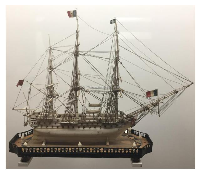
Third rate warship with two gun decks, 88 cannon and figurehead. The rather small ship model is built from larger pieces of bone, there are no planks in the underwater hull.
